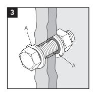
Attach the frame using bolts, nuts and washers. Through-holes must be sealed using sealant or sealing washers (A).
