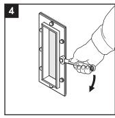
Tighten the fasteners crosswise in small steps. The gasket shall be compressed at least by 80%.
