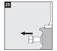
The visible part of the screw will increase during tightening.
