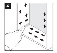
Lubricate the sealing surfaces of the frame with Roxtec Lubricant. Lubricate the corners thoroughly.
