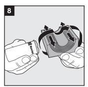
Lubricate the sealing surfaces.
