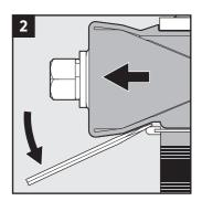
Remove the wedge by lifting it over the stayplate using a flat tool.
