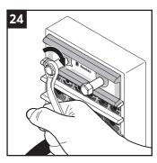
Tighten the screws alternately in small steps until full mechanical stop (~25-30 Nm). Protruding excess lubricant indicates a tight seal.
