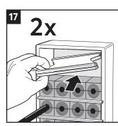
Before inserting the final row of modules, insert two stayplates.
