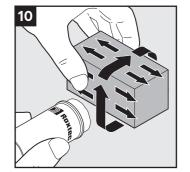
Lubricate solid modules on the sealing surfaces.
