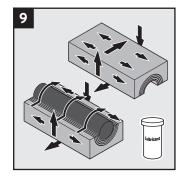
Lubricate the sealing surfaces of any spare module. Do not remove the core.
