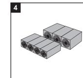
Keep the module rows sorted until reinstallation. If a module needs to be replaced, all modules in that row must be replaced.
