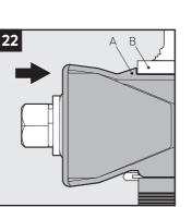
Ensure that the wedge is secured within the stayplate edges. The stop edge (A) is flush to the frame (B).
