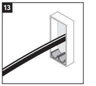
Cables/pipes shall go in parallel with the frame.
