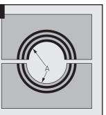
The number of layers may not differ (A) by more than one between the corresponding module halves.
