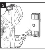
Tack weld the frame to the structure. Pre-heating of the frame to approx. 50°C is recommended.
