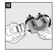
Lubricate the sealing surfaces of all modules with Roxtec Lubricant.
