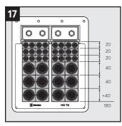
Consider the packing height of the frame. This is an example of a packing plan.
