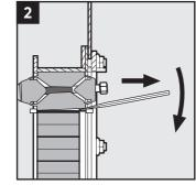
Insert a flat tool between the wedge and the stayplate to simplify removal of the wedge.
