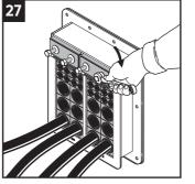
Tighten the screws alternately in small steps until full mechanical stop (~25-30 Nm). Protruding excess lubricant indicates a tight seal.
