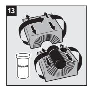
Lubricate the sealing surfaces of the spare modules. Do not remove the core.
