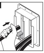
Insert cables/pipes straight through the frame.
