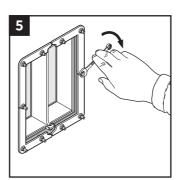
Tighten the nuts crosswise in small steps. Recommended torque 4 Nm.
