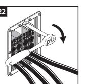
Use a Roxtec pre-compression tool to make space for the wedges, if required.
