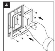
Attach the four parts of the counter frame from the inside of the cabinet.
