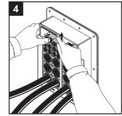
Lift the stayplate and push out the upper module from the front side
