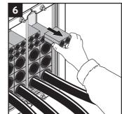
Continue to remove the modules by pulling them out from the backside of the frame.
