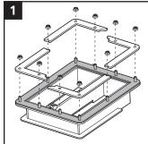
Remove the four parts of the counter frame.
