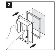
Insert the frame from the outside of the cabinet with the gasket in between.
