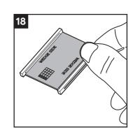
Orientate the stayplate so the text "wedge side" faces the wedge.
