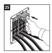
Insert the wedges from the inside of the openings until stop. The wedges can be placed with the screwhead facing either into or out of the opening.
