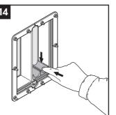
Insert the modules from the back side of the transit according to
