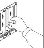
Lubricate the sealing surfaces of the frame. Lubricate the corners thoroughly.
