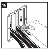
Place the corresponding module half on top. Continue to fill the transit considering your packning plan.
