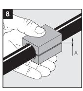
Achieve a gap of 0.1-1.0 mm (A) between the module halves by peeling off layers.
