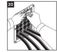
Lift the upper stayplate and insert the last module underneath it.
