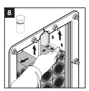
Lubricate the exposed surfaces, especially in the corners. Continue the reinstallation
