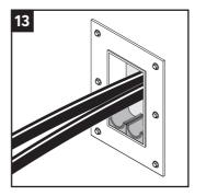
Cables/pipes shall go in parallel with the frame.
