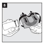
Lubricate the sealing surfaces with Roxtec Lubricant.
