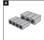
Keep the module rows sorted until reinstallation. If a module needs to be replaced, all modules in that row must be replaced.
