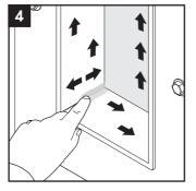
Lubricate the sealing surfaces of the frame. Lubricate the corners thoroughly.
