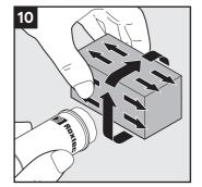
Lubricate solid modules on the sealing surfaces.
