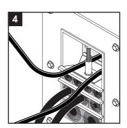
Partially installed openings shall be compressed if left unattended. Excess lubricant is a sign of good compression.
