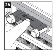
Attach the wedge clip. The wedge clip verifies correctly tightened wedge
