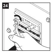
Tighten the screws alternately in small steps until full mechanical stop (~25-30 Nm). Protruding excess lubricant indicates a tight seal.
