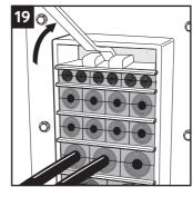
A Roxtec pre-compression tool can be used to make room for the wedge, if necessary.
