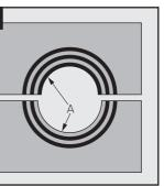
The number of layers may not differ (A) by more than one between the corresponding module halves.
