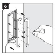
Attach the two parts of the counter frame from the inside of the cabinet.
