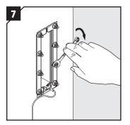
Tighten the nuts crosswise in small steps. Recommended torque 4 Nm. Do not overtighten the nuts.
