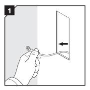
Route the protective bonding conductor through the aperture.
