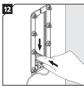
Push the modules in place. Ensure that the module rests against the stopping edge at the front.
