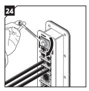
Tighten the screw of the compression unit until full stop. Do not exceed 20 Nm.
