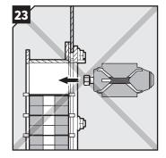
Do not install the compression unit with the screwhead facing the frame.
