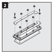
Remove all nuts and the two parts of the counter frame.
