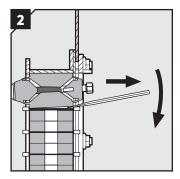
Insert a flat tool between the compression unit and the stayplate to simplify removal of the compression unit. Roxtec special tools are available.
