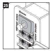
Visible excess assembly gel Ex is a sign of good compression. Make sure that all modules are placed correctly and fully inserted after compression.
