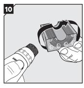
Lubricate all modules for the frame thoroughly with Roxtec Assembly Gel Ex, both the inside and the outside surfaces.
