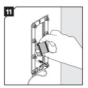
Insert the modules from the back side of the transit according to your installation plan. Start with the largest modules.
