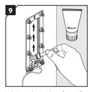
Lubricate the inside surfaces of the frame all around with Roxtec Assembly Gel Ex, especially into the corners.
