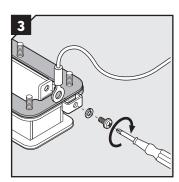
Attach a protective bonding conductor to the frame earthing terminal.
