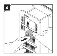
Lift the stayplate and push out the upper module from the front side.
