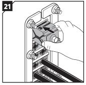
Insert the compression unit until stop. The compression unit can be inserted from any direction.
