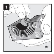
Adapt modules, which are to hold cables, by peeling off layers until you reach the gap seen in pic. 3. The number of layers may not differ by more than one between the halves.
