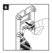
Continue to remove the modules by pulling them out from the backside of the frame.
