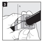
Achieve a 0.1-1.0 mm (A) gap between the two halves when held against the cable.
