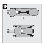
Ensure that the compression unit is fully uncompressed (A) by untightening the screw of the compression unit before inserting it
