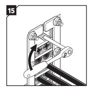
Use a Roxtec pre-compression tool to make space for the compression units if required.
