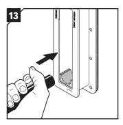
Insert the cables through the frame.
