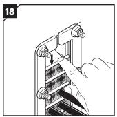
Drop the stayplate on top of the last row of modules. Make sure the combinations of modules equal the 160 mm packing space. See example on page 2.
