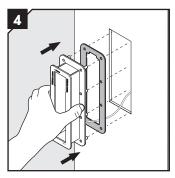
Insert the HD 16 Ex frame from the outside of the cabinet. Ensure that the gasket is placed between the frame and the cabinet.
