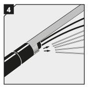
Cut the armor at the mark with a tool recommended by the cable manufacturer. Make sure not to damage the
