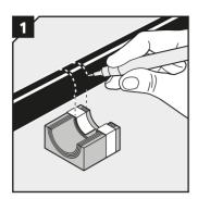
On the cable, make two marks where outer jacket is to be cut.
