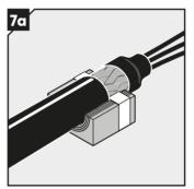
Make sure that the shrink tube is completely outside the module.
