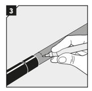
Mark where the armor is to be cut. The remaining armor shall accommodate both the braid of the module and the piece of cable jacket according to step 6.
