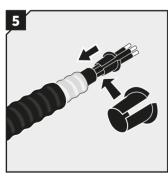
When required for inner conductor protection, fit an anti-short bushing or similar at the end cut of the cable armor.
