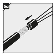
Cover the end of the cable braid with a piece of shrink tube.
