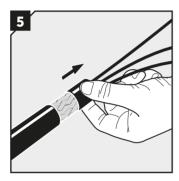
Pull the piece of cable jacket away to cover the end of the cable braid. The exposed cable braid shall accommodate both the braid and the remaining rubber of the module.
