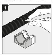
On the cable, mark where outer jacket is to be removed.
