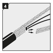
Cut the cable braid at the mark with a tool recommended by the cable manufacturer. Make sure not to damage the cables.
