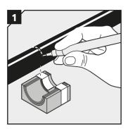
On the cable, mark where outer jacket is to be cut.
