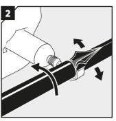
Cut the outer jacket at the mark with a tool recommended by the cable manufacturer. Make sure not to damage
