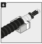
Make sure that the armor extends beyond the edge of the module and that the anti-short bushing is in place where applicable.
