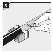
Mark where the braid is to be cut. The remaining cable braid shall accommodate both the braid of the module and the piece of shrink tube according to step 7a or 7b.
