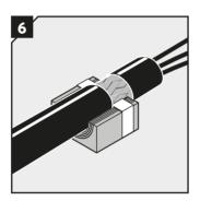
Make sure that the piece of cable jacket is completely outside the module.
