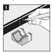
On the cable, make two marks where the outer jacket is to be cut.
