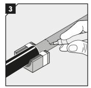
Mark where the armor is to be cut. The remaining armor shall accomodate both the braid of the module and the piece of shrink tube according to step 7a or 7b.
