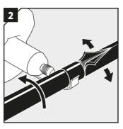
Cut the outer jacket at the two marks with a tool recommended by the cable manufacturer. Make sure not to damage the cable braid. Remove excess jacket.
