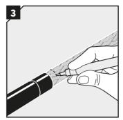
Mark where the cable braid is to be cut. The remaining cable braid shall accomodate both the braid of the module and the piece of cable jacket according to step 6.
