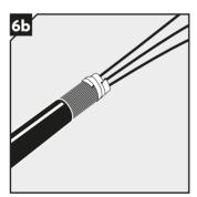
Make sure that the tape is completely outside the module.
