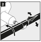
Cut the outer jacket at the two marks with a tool recommended by the cable manufacturer. Make sure not to damage the cable armor. Remove excess jacket.
