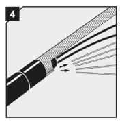
Cut the armor at the mark with a tool recommended by the cable manufacturer. Make sure not to damage the cables.
