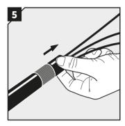
Pull the piece of cable jacket away to cover the end of the armor. The exposed armor shall accommodate both the braid and the remaining rubber of the module.
