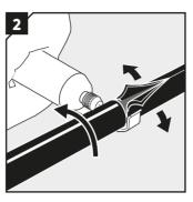
Cut the outer jacket at the mark with a tool recommended by the cable manufacturer. Make sure not to damage the cable braid.
