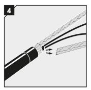
Cut the braid at the mark with a tool recommended by the cable manufacturer. Make sure not to damage the cables.
