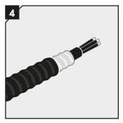
Cut the cable armor at the mark with a tool recommended by the cable manufacturer. Make sure not to damage the cables.
