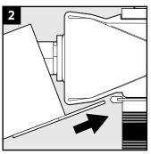
Insert the wedge puller between the wedge and the stayplate
