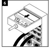
Tighten the nut of the wedge puller to remove the wedge.
