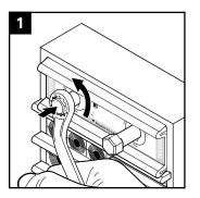
Turn the bolts counter-clockwise to release the compression. Make sure to leave approximately 6 mm between the wedge and the bolt heads to make room for the wedge puller hook.
