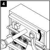
Place the wedge hook behind the bolt heads. Turn the bolts counter-clockwise to secure the wedge puller hook behind the bolt heads.
