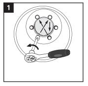
Loosen the screws alternately in small steps. Do not unscrew the two top screws completely.
