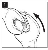
Untighten the nut and remove the SLA sleeve
