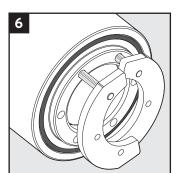
Place the fittings one above the other to allow insertion into the aperture.
