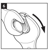
Tighten the nut firmly until the O-ring is compressed and the sleeve is flush with the structure. Prevent the sleeve from rotating by using another spanner.
