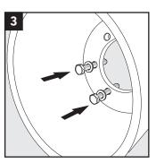
Insert two of the screws in the SLA sleeve.
