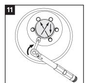
Tighten the screws crosswise in small steps until the O-ring is compressed and the sleeve is flush with the structure.
