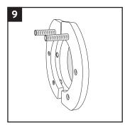
With the sleeve in position, tighten the two screws and align the holes in the sleeve with the threaded holes in the fittings.
