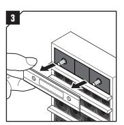
Remove the fitting of the top packing.
