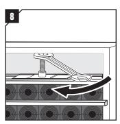
Loosen the compression plate nut.
