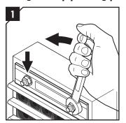
Turn the nuts counter-clockwise to release the compression.
