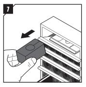
Remove the center piece of the top packing.
