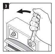
Loosen the nuts on the top packing to make room for the adapter.
