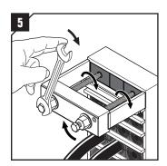
Attach the top packing puller to the top-packing. Attach evenly to the two bolts.
