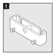
Use this Roxtec adapter with the top packing puller to remove top packings of other brands.
