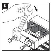
Turn either one of the two larger nuts clockwise on the puller. The top packing will now be pulled from the frame
