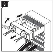
Turn either one of the two larger nuts clockwise on the puller. The top packing/wedge will now be pulled from the frame.
