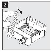
Mount the adapter to the Top packing puller.
