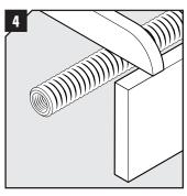
Locate the two threaded holes on the Top packing puller.
