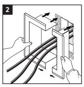
Use a openable GE frame for pre routed cables.
