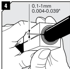
Try to achieve a 0.1–1 mm gap between the two halves when held against the cable/pipe. Use the Ex Gap Gauge.
