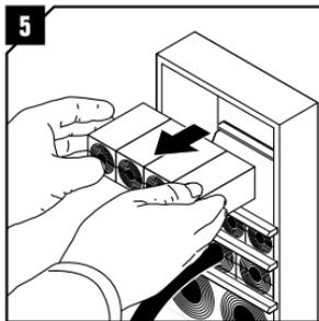
5 Remove the modules required. Keep the rows sorted until it is time to re-install the transit. If a module is damaged or replaced, all modules in that row must be replaced.
