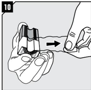
Remove the plastic film! Keep the tape clean. **Note:** Plastic film and paper must be removed on spares and solid modules.
