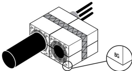
All modules should be of the same type, Roxtec RM BG Ex, in each opening. Please note the markings on the module end.
