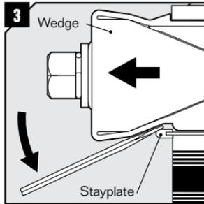
3 Insert a flat tool between the wedge and the stayplate to simplify removal of the wedge. Roxel special tools are available.
