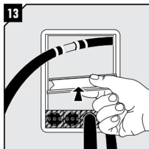
Insert a stayplate on top of every finished row of modules. Make sure the stayplate is clean.
