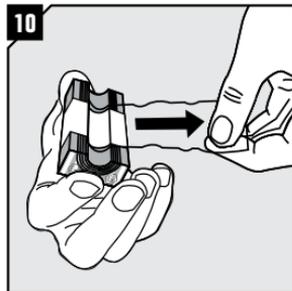
Remove the plastic film! Keep the tape clean. **Note:** Plastic must be removed on spares as well.
