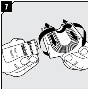
Lubricate the modules thoroughly with Roxel Lubricant, both the inside and outside faces.
