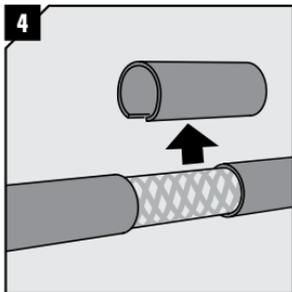
4 Remove the outer sheath and any plastic foil. Make sure cable screen is clean.
