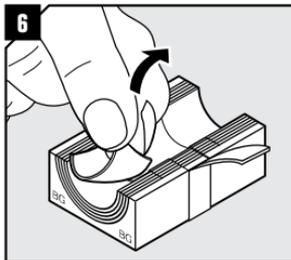
Adapt layers on both module halves to fit outer jacket.
