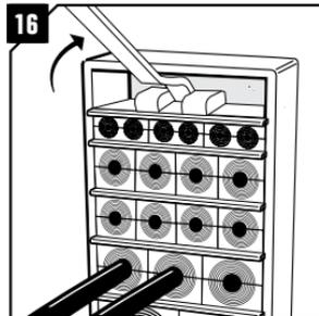
If there is not enough room for the EMC wedge, insert the optional Roctec pre-compression tool.
