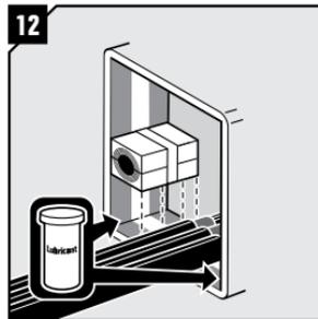
Lubricate the frame and the areas that will be in contact with the rubber of the modules. Avoid excess lubricant on areas in contact with the braid.
