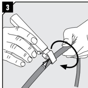
**3** Cut the outer sheath with a tool of your choice. Make sure not to damage the cable screen.
