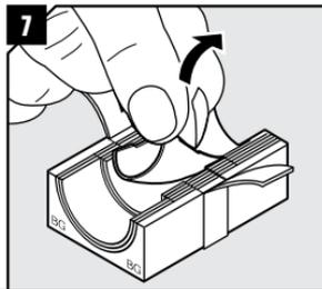
Adapt layers on both module halves to fit cable screen/armor.
