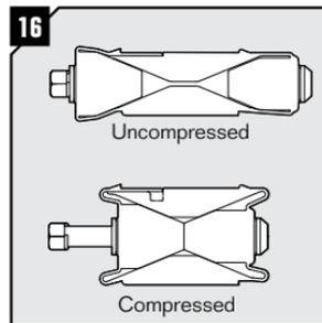
Ensure that the wedge is fully uncompressed by untightening the screws of the wedge before inserting it.
