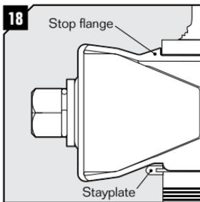
Oriente the wedge so the face marked "Stayplate this side" faces a stayplate. Insert the wedge to the stop flange. Ensure that the wedge is accommodated and secured by the stayplate.
