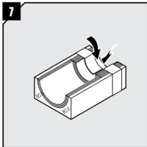
Fold the braid tightly inside the module.
