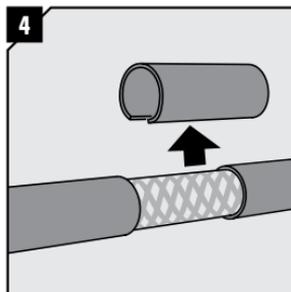
Remove the outer sheath and any plastic foil. Make sure cable screen is clean.
