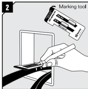
**2** On the cable, mark the module position and where the outer sheath is to be removed.
