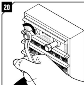
Tighten the screws alternately until full stop, approx 20 Nm (15 ft.lb.).
