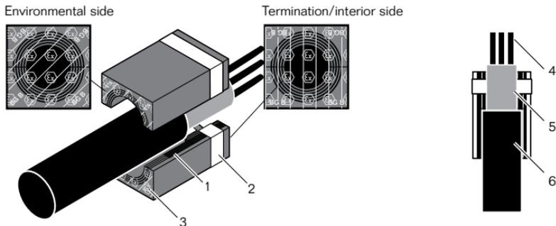
1. Multidiameter™ – adapts to cables and pipes of different sizes through removable layers
