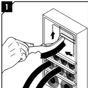
1 Make sure that the inside surfaces of the exposed packing space are free from dirt or dust.
