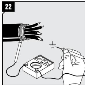
Verify earth continuity from each cable armor/screen to earth. Use a suitable instrument.
