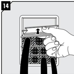
Before inserting the final row of modules, insert two stayplates together.
