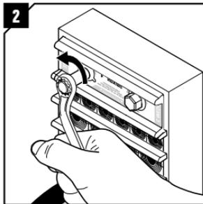
2 Release the compression by loosening the screws alternately to full stop. Do not exceed 20 Nm (15 ft.lb.).
