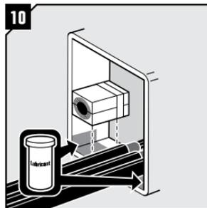
Lubricate the frame on the areas that will be in contact with the rubber of the modules. Avoid excess lubricant on areas in contact with the braid.
