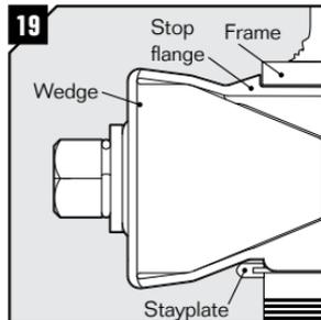
Orienteate the EMC wedge so the face marked "Stayplate this side" faces a stayplate. Insert the wedge to the stop flange. Ensure that the wedge is accommodated and secured by the stayplate.
