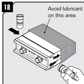
Lubricate the short sides of the EMC wedge only.
