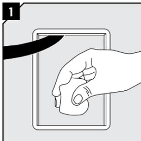
**1** Clean the empty frame from paint, dirt, etc. to secure good electrical conductivity.
