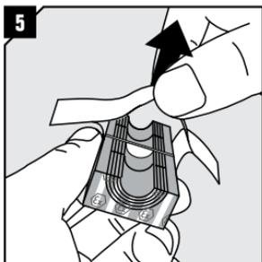
Remove the protection paper from the modules and fold back the tape.
