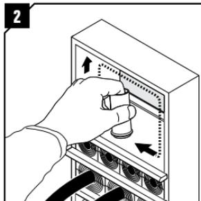
2 Lubricate the inside surfaces all around with Roxtec Lubricant, especially into the corners.
