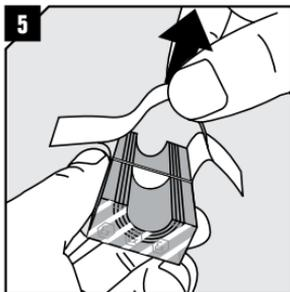
5 Remove the protection paper from the modules and fold back the tape. It is not necessary to remove the paper from spare modules.
