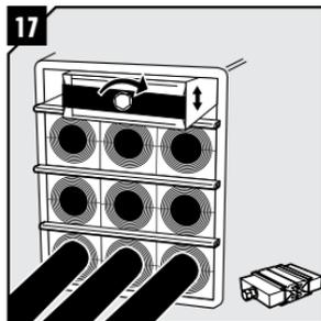
Pre-compress by using Roxel pre-compression wedge.
