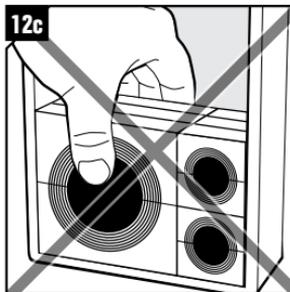
It is not permitted to stack smaller modules on top of each other.
