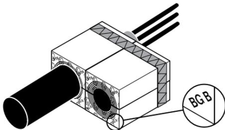
All modules should be of the same type, Roctec RM BG B Ex, in each opening and placed in the same direction. Please note the markings on the module end.
