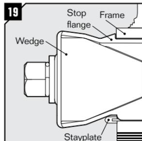
Orientate the EMC wedge so the face marked "Stayplate this side" faces a stayplate. Insert the wedge to the stop flange. Ensure that the wedge is accommodated and secured by the stayplate.
