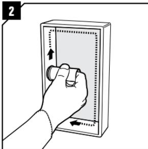
Lubricate the inside faces of the frame with Roxel lubricant. Make sure to lubricate into the corners.
