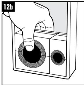
When inserting larger modules, pay attention so that every row of modules is separated by a stayplate. It is not permitted to stack smaller modules on top of each other.
