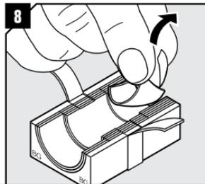
**For alternative 1:** Adapt layers on both module halves to fit outer jacket.
