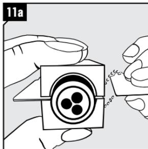
Measure the gap with the Ex Gauge by holding blade one in one gap and checking the other with blade two.
