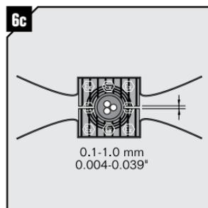
When checking without the gauges there shall be a gap of 0.1-1.0 mm (0.004"-0.039"). If not, repeat 6a-b. The halves may not differ by more than one layer. Make sure the screen is in good contact with the module.
