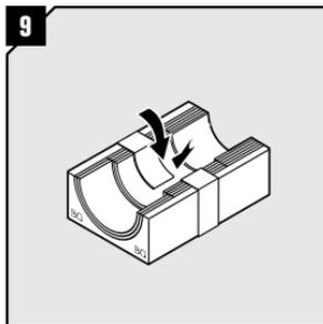
Fold the braid tightly inside the module.
