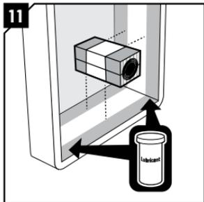
Lubricate the frame and its corners on the areas that will be in contact with the rubber of the modules. Do not lubricate the areas that will be in contact with the tape.
