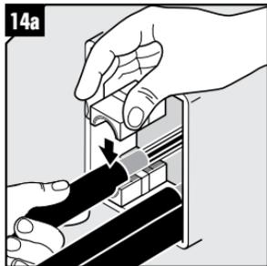
Insert the module halves directly under and on top of the cables. Do not slide them in.
