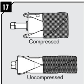
Ensure that the EMC wedge is fully uncompressed by untightening the screws of the wedge before inserting it.
