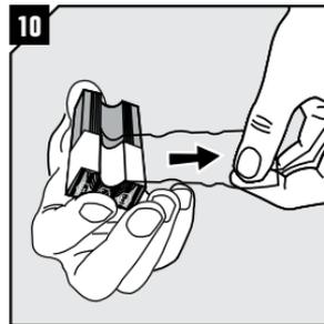
Remove the plastic film! Keep the tape clean. **Note:** Plastic and paper must be removed on spares and solid modules.
