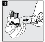
Remove the plastic film! Keep the tape clean. **Note:** Plastic and paper must be removed on spares and solid modules.
