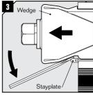
Insert a flat tool between the wedge and the stayplate to simplify removal of the wedge. Roxtec special tools are available.
