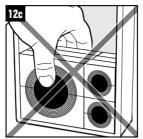
It is not permitted to stack smaller modules on top of each other.
