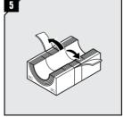
Remove the core and fold back the braid on modules.
