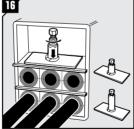
During installation, you can use the pre-compression S or L tool to make room.
