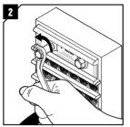
Release the compression by loosening the screws alternately to full stop. Do not exceed 20 Nm (15 ft.lb.).
