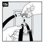
Place cables, according to your transit plan, in the module halves. Place corresponding module half directly on top. Do not slide them in.
