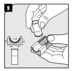
Lubricate all modules sparsely with Roxtec Lubricant on inside and outside rubber surfaces only. Do not lubricate the film.
