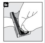
Adapt layers to fit outer jacket. (Fig 1 section A).
