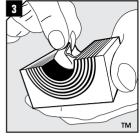
Adapt modules which are to hold cables or pipes by peeling off layers. The halves may not differ by more than one layer.
