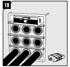
Pre-compress by using Roxtec precompression wedge.
