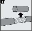
Remove the outer sheath and any plastic foil. Make sure the cable screen is clean.
