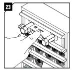
Attach the Wedge Clip to the EMC wedge screws to complete the installation.
