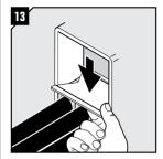
Insert a stayplate on top of every finished row of modules. Make sure the stayplate is clean.
