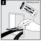
On the cable, mark the module position and where the outer sheath is to be removed.
