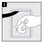
Clean the empty frame from paint, dirt, etc. to secure good electrical conductivity.
