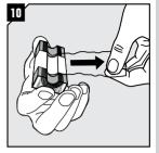
Remove the plastic film! Keep the tape clean. **Note**: Plastic must be removed on spares as well.
