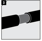
Alternative 1: Remove a length of outer jacket to accommodate the module braid to ensure full conductivity. Remove any protection tape or plastic if applicable.
