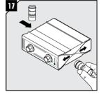
Lubricate the short sides of the wedge.
