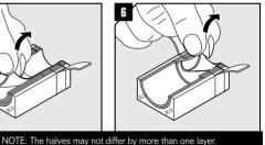
Adapt layers on both module halves to fit cable screen/armor.
