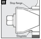
Orientate the wedge so the face marked "Stayplate this side "faces a stayplate. Insert the wedge to the stop flange. Ensure that the wedge is accommodated and secured by the stayplate.
