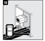
Lubricate the frame on the areas that will be in contact with the rubber of the modules. Avoid excess lubricant on areas in contact with the braid.
