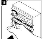
Tighten the screws alternately until full mechanical stop, approx 20 full revolutions per screw. Do not exceed 20 Nm (15 ft.lb.).
