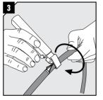
Cut the outer sheath with a tool of your choice. Make sure not to damage the cable screen.
