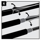
Alternative 2: Remove a length of outer jacket to accommodate the module braid to ensure full conductivity. Remove any protection tape or plastic if applicable.
