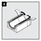
Remove the core and fold back the braid on modules.
