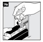
Insert the module halves directly under and on top of the cables. Do not slide them in.
