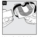
Lubricate all modules for the frame thoroughly, both the inside and the outside surfaces. Avoid excess lubricant on the braid.
