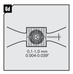
When checking without the gauges there shall be a gap of 0.1-1.0 mm (0.004"-0.039"). If not, repeat 6a-c. The halves may not differ by more than one layer. Make sure the screen is in good contact with the module.
