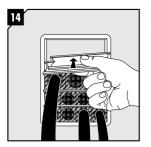
Before inserting the final row of modules, insert two stayplates together.
