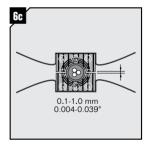
When checking without the gauges there shall be a gap of 0.1-1.0 mm (0.004"-0.039"). If not, repeat 6a-b. The halves may not differ by more than one layer. Make sure the screen is in good contact with the module.
