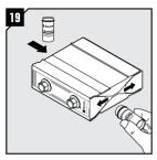
Lubricate the short sides of the wedge.
