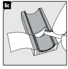
Adapt vertical screen to fit cable screen. (Fig 1:C).
