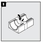
Fold the braid tightly inside the module.
