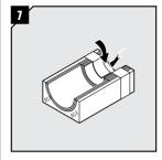
Fold the braid tightly inside the module
