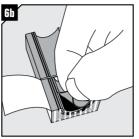
Adapt layers to fit cable screen. (Fig 1:B).
