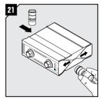
Lubricate the short sides of the wedge.
