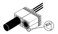
All modules should be of the same type, Roxtec RM BG B Ex, in each opening and placed in the same direction. Please note the markings on the module end
