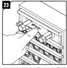
Attach the Wedge Clip to the EMC wedge screws to complete the installation.
