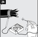
Verify earth continuity from each cable armor/screen to earth. Use a suitable instrument.
