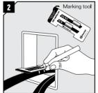
On the cable, mark the module position and where the outer sheath is to be removed.
