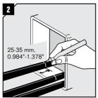
On the cable, mark where outer sheath and armor, if applicable, are to be removed.
