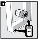
Lubricate the frame and its corners on the areas that will be in contact with the rubber of the modules. Do not lubricate the areas that will be in contact with the tape.
