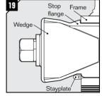
Orientate the EMC wedge so the face marked "Stayplate this side" faces a stayplate. Insert the wedge to the stop flange. Ensure that the wedge is accommodated and secured by the stayplate.
