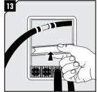
When inserting larger modules, pay attention so that every row of modules is separated by a stayplate. It is not permitted to stack smaller modules on top of each other.
