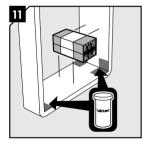
Lubricate the frame and its corners on the areas that will be in contact with the rubber of the modules. Do not lubricate the areas that will be in contact with the tape.
