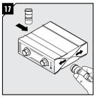
Lubricate the short sides of the wedge.
