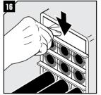
Separate the two stayplates and insert the final row of modules between the stayplates. Drop the upper stayplate on top of the modules
