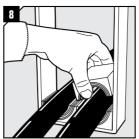
Insert the modules according to your transit plan. Start with the largest modules.
