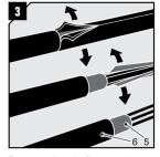
Remove a length of outer jacket to accommodate the module braid to ensure full conductivity. Remove any protection tape or plastic if applicable.
