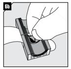
Adapt layers to fit cable screen. (Fig 1section B).
