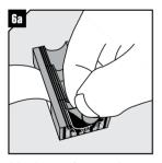
Adapt layers to fit outer jacket. (Fig 1 section A).
