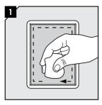
Clean the empty frame from paint, dirt, etc, to secure good electrical conductivity.
