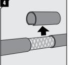
Remove the outer sheath and any plastic foil. Make sure cable screen is clean.
