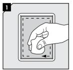
Clean the empty frame from paint, dirt, etc, to secure good electrical conductivity.
