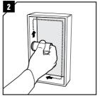
Lubricate the inside faces of the frame with Roxtec lubricant. Make sure to lubricate into the corners.
