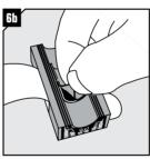
Adapt layers to fit cable screen. (Fig 1section B).
