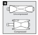
Ensure that the wedge is fully uncompressed by untightening the screws of the wedge before inserting it.
