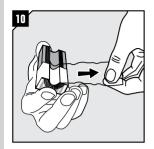
Remove the plastic film! Keep the tape clean. **Note:** Plastic film and paper must be removed on spares and solid modules.
