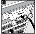
Attach the Wedge Clip to the wedge screws to complete the installation.
