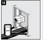
Lubricate the frame and the areas that will be in contact with the rubber of the modules. Avoid excess lubricant on areas in contact with the braid.
