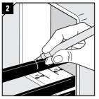
On the cable, mark where outer jacket and armor, if applicable, are to be removed (see alternatives 1 or 2).
