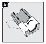
Fold the tape on the other side tightly inside the module half. There must be no air-pockets.
