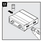
Lubricate the short sides of the wedge.
