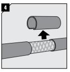
Remove the outer sheath and any plastic foil. Make sure cable screen is clean.
