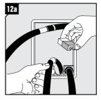
Place cables, according to your transit plan, in the module halves. Place corresponding module half directly on top. Do not slide them in.
