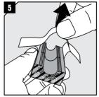
Remove the protection paper from the modules and fold back the tape. It is not necessary to remove the paper from spare modules.
