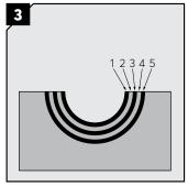
The indicator shows which layer to keep. Remove one layer less than the indicated number.
