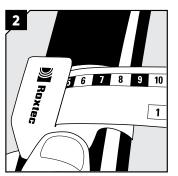
The indicator shows which size of module to use as well as how to adapt it to the cable.
