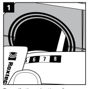
To verify the adaption of modules: Fold the indicator around the cable. Read the indicator and count backwards how many layers should remain.
