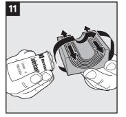
Lubricate the sealing surfaces of the modules.
