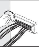
Tighten the screw of the compression unit to the specified
