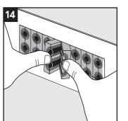
To simplify the insertion of the last module, angle the module halves and press them into the frame simultaneously.
