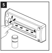
Clean and lubricate the sealing surfaces of the frame with Roxtec Lubricant, especially in the corners.
