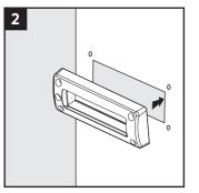
Insert the frame into the opening.
