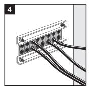
For EzEntry 16, use the counter flange (article no. 2CV000000016) if the thickness of the structure is 2 mm or less.
