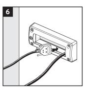
Insert the cables straight through the frame.
