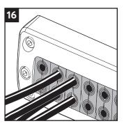
Excess lubricant shall be visible, and is a sign of good compression.
