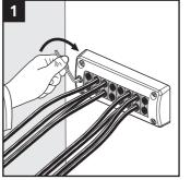
Untighten the screw of the integrated compression unit.
