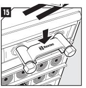
Attach the Wedge Clip to the wedge bolts to check that the wedge is properly tightened.
