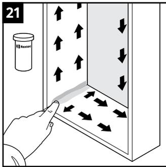
Lubricate the inside surfaces of the frame and especially its corners.
