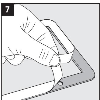
Remove the protection foil from the gasket.
