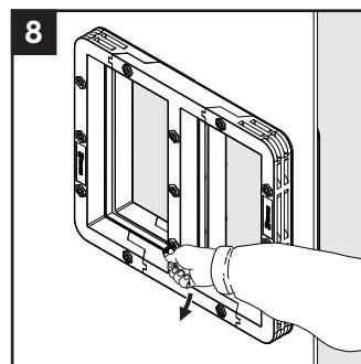
Tighten the screws crosswise in small steps to 7 Nm.
