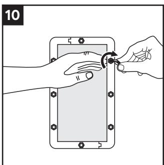
Insert and tighten all the bolts to 7 Nm.
