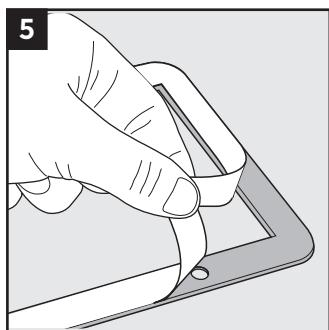
Remove the protection foil from the gasket.
