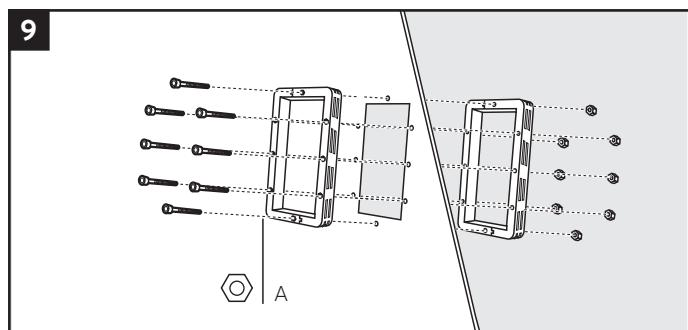
Place the frame with the gasket side against the wall and insert all bolts and nuts. Hexagonal bolt holes (A) must point outwards, away from the wall structure.
