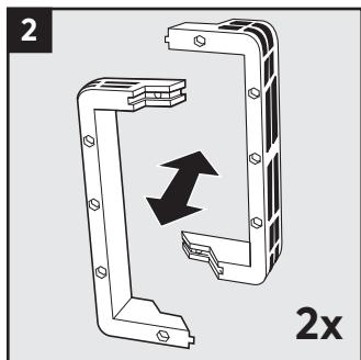
Divide the frame into two frame parts.
