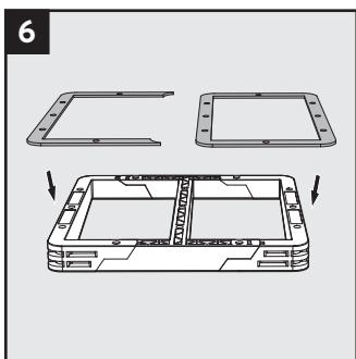
Attach the adhesive gasket parts on the frame side with the round holes, which should face the structure.
