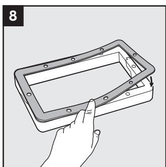
Attach the adhesive gasket on the frame side with the round holes, which should face the structure.
