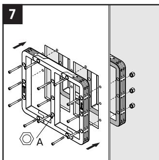
Place the frame with the gasket side against the wall and insert all bolts and nuts. Hexagonal bolt holes (A) must point outwards, away from the wall structure.
