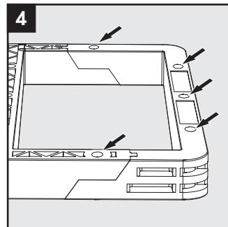
Lay the frame with the un-recessed holes upward.
