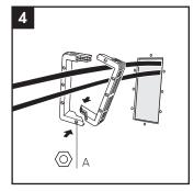
If cables are pre-routed, reconnect the frame parts around the cables. Hexagonal bolt holes (A) must point outwards, away from the wall structure.
