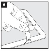
Remove the protection foil from the gasket.
