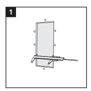
Make or verify an aperture. Structure thickness shall be between 5 - 8 mm.
