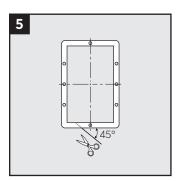
If cables are pre-routed, you will have to cut the gasket in a 45° angle, on the short side, to be able to mount it.
