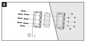
Place the frame with the gasket side against the wall and insert all bolts and nuts. Hexagonal bolt holes (A) must point outwards, away from the wall structure.
