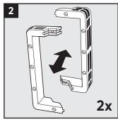
Divide the frame into two frame parts.
