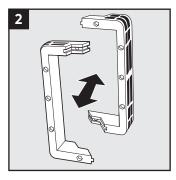
Divide the frame into two frame parts.
