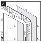
The hexagonal holes shall face outwards.
