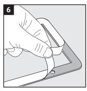
Remove the protection foil from the gasket.
