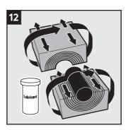
Lubricate the sealing surfaces of the spare modules.
