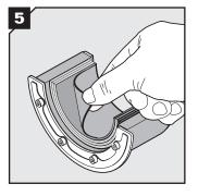
Adapt the seal by peeling off layers from the halves until you reach the gap seen in step 6. The number of layers may not differ by more than one between the halves.
