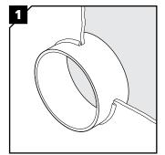
Weld the sleeve to the cabinet/wall. Welding instructions available on www.roxtec.com
