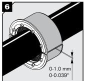
Achieve a 0-1.0 mm gap between the two halves when held against the cable/pipe.
