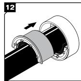
Insert the halves into the sleeve.
