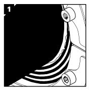
Excess lubricant shall be visible after compression.
