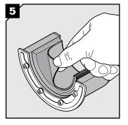
Adapt the seal by peeling off layers from the halves until you reach the gap seen in step 6. The number of layers may not differ by more than one between the halves.
