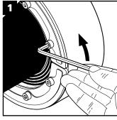
Release the compression by loosening the screws alternately.
