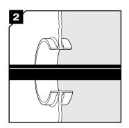
Feed the cable through the opening. The cable/pipe shall go straight and centered through the sleeve.
