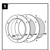
Use the sleeve as template for the drilling of the screw holes. Drill Ø = 8.5 mm.
