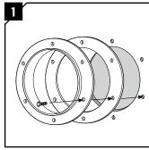
Use the sleeve as template for the drilling of the screw holes. Drill  $\emptyset$  = 8.5 mm.
