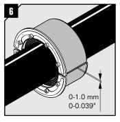
Achieve a 0-1.0 mm gap between the two halves when held against the cable/pipe.
