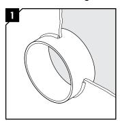
Weld the sleeve to the cabinet/ wall. Welding instructions available on www.roxtec.com
