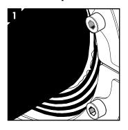
Excess lubricant shall be visible after compression.
