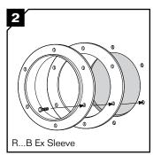
Sleeve for bolting. Use the sleeve as template for the drilling of the screw holes. Drill  $\emptyset = 8.5$  mm.
