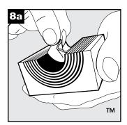
Adapt the modules which are to hold cables or pipes by peeling off layers. The halves may not differ by more than one layer.
