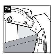
For pre-routed cables, use the RO (openable) frame. Disassemble and open the RO frame and wrap it around the cables.
