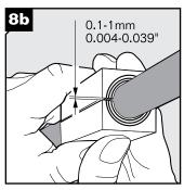
Try to achieve a 0.1–1.0 mm gap between the two halves when held against the cable/pipe.
