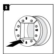
Lubricate the outside of the R frame sparsely. Insert the frame into the hole. Push the front fittings of the frame to the sides.
