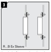
Attach the frame to the cabinet/wall using bolts and nuts. The rubber gasket shall be placed between frame and cabinet/wall.
