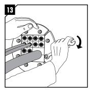
Tighten the nuts crosswise until the frame is sealed.
