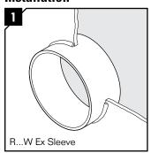
Sleeve for welding. Weld the sleeve to the cabinet/wall. Welding instructions available on www.roxtec.com
