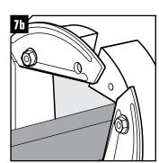
For pre-routed cables, use the RO (openable) frame. Disassemble and open the RO frame and wrap it around the cables.
