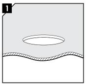
Make a hole for the sleeve, according to the recommended hole cut. See table above.
