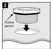
Make sure the rubber gasket is in place and insert the sleeve.
