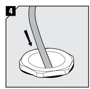
Insert the cable through the sleeve.
