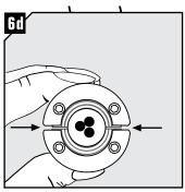
When checking without the gauge, there shall be a visual gap.
