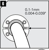
Achieve a 0.1-1 mm gap between the halves when testing against the cable.
