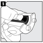
Adapt the seal to the cable by removing layers from the halves. The halves may not differ by more than one layer.
