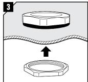
Fit the nut from inside, tighten and fasten the sleeve.
