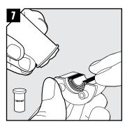
Lubricate thoroughly on the inside surfaces and sparsely on the outside of the seal.
