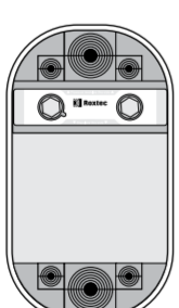
For frames with 40 mm inner radius, place one RM 40 and two RM 20 modules between the RC modules.
