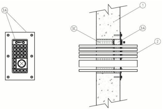
1. **Wall Assembly** — Min 5 in. (127 mm) thick lightweight or normal weight (100-150 pcf or 1600-2400 kg/m³) concrete. Wall may also be constructed of any UL Classified **Concrete Blocks\***. Rectangular opening to have dimensions which are max 1/4 in. (6 mm) greater than the width and height of the firestop device frame (Item 3A), excluding mounting flanges. Max dimension of opening is 6 in. (152 mm) wide by 12 in. (305 mm) high (G 8X1 Device).
